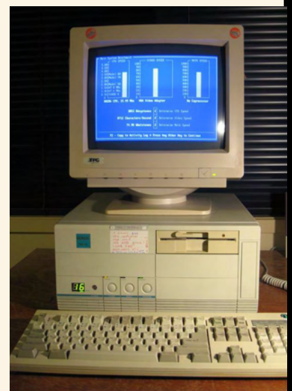
Personal computer with 80286 processor and 5 1/4" floppy disk drive
