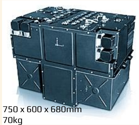
Argon-16: first board computer of the Soviet Soyuz T-2 in 1980
